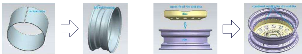
Figure 4: Welding process in rim manufacturing
